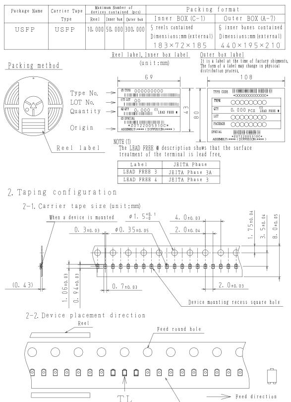
Those with one electrode terminal on the feed hole side ..... TL
