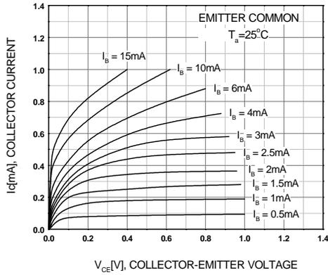
Figure 1. Static Characteristic
