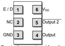
Terminations as viewed from the Top NOTE: XPRESSO-ULTRA LVDS XOs are designed to fit on Industry Standard, 6 pad layouts
