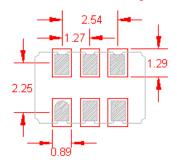
**NOTE:** XPRESSO-ULTRA LVDS XOs are designed to fit on Industry Standard, 6 pad layouts
