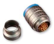
Series 881 threaded coupling, cable plug with solder cup contacts feature threadon rear adapters allowing access to solder cup contacts. Install cable shield braid directly to connector with Band-Master Micro band. Three contact sizes are available with current ratings of 5A, 3A and 1A. Aluminum or stainless steel housings, thermoplastic insulators. Ultraminiature SuperFly® connectors are ideal for soldier systems and other applications where ruggedness and field repairability is required.
