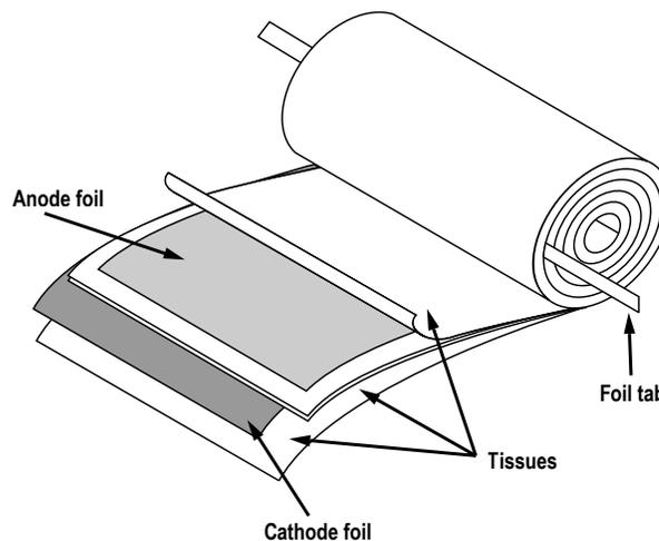
The winding is assembled to the capacitor aluminum can and to the aluminum lid. The can is filled with electrolyte and the winding is impregnated during a vacuum treatment. The capacitor is sealed. Throughout the process, all materials inside the housing must be maintained at the highest purity and be compatible with the electrolyte.
