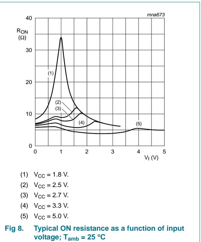
**Fig 8. Typical ON resistance as a function of input voltage; T<sub>amb</sub> = 25 °C**
