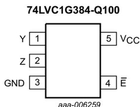
Fig 4. Pin configuration SOT353-1 and SOT753
