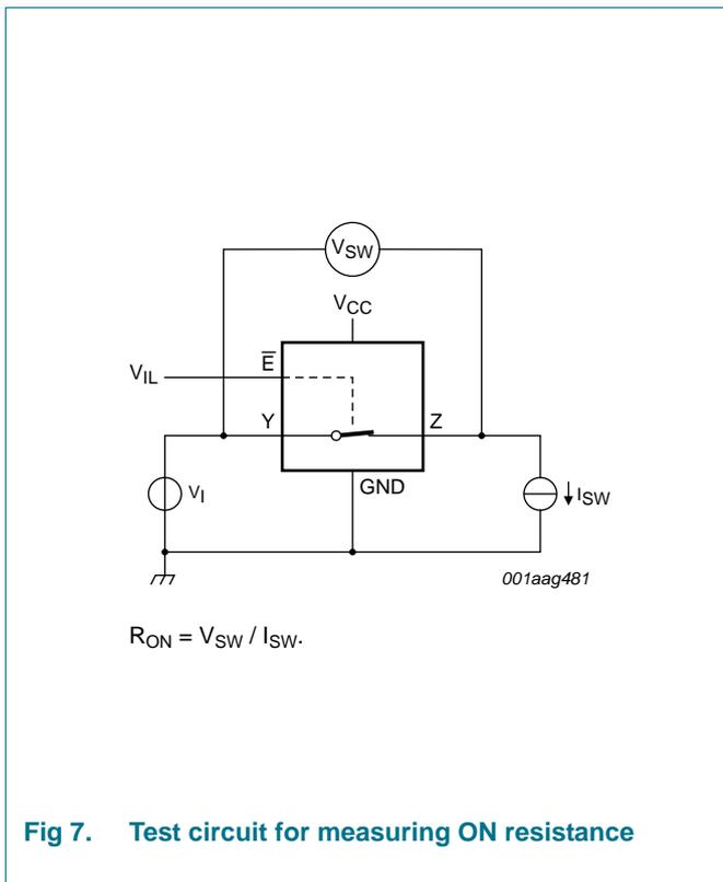
**Fig 7. Test circuit for measuring ON resistance**
