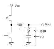
Fig.28 Output capacitor
