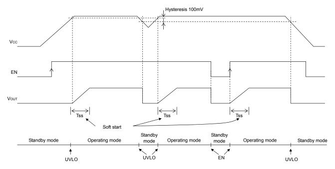
Fig.24 Soft start, Shutdown, UVLO timing chart
