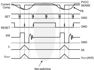
Fig.23 SLLM<sup>TM</sup> switching timing chart
