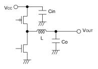
Fig.29 Input capacitor
