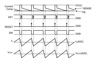
Fig.22 PWM switching timing chart
