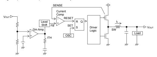
Fig.21 Diagram of current mode PWM control
