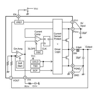
Fig.2 BD9111NV Block Diagram
