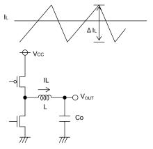
Fig.27 Output ripple current
