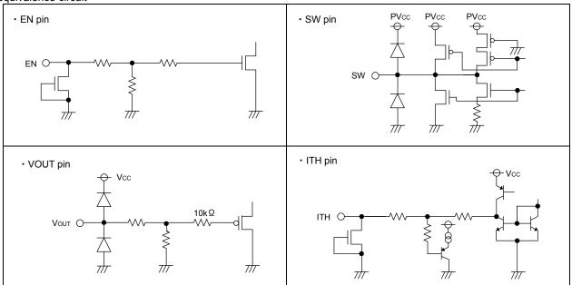
Fig.34 I/O equivalence circuit
