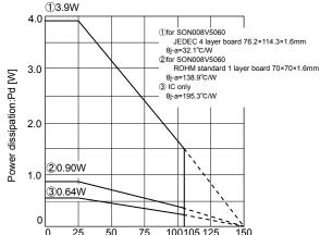
Ambient temperature:Ta [°C] Fig.26 Thermal derating curve (SON008V5060)
