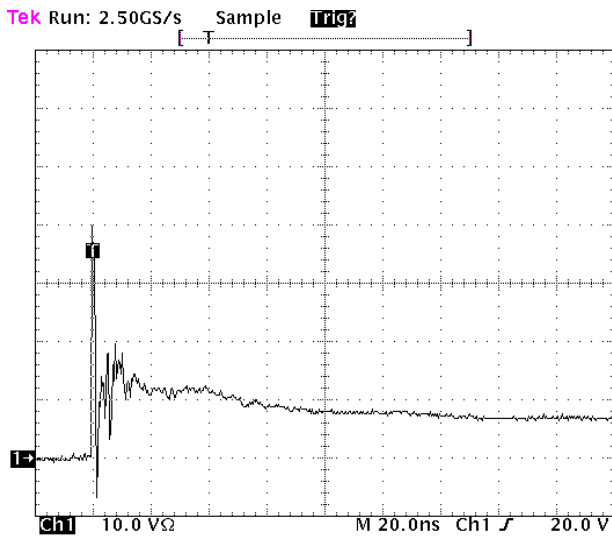
Figure 22. D+ & D- Clamping Voltage Screenshot Positive 8 kV Contact per IEC61000-4-2
