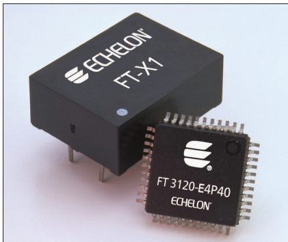
FT 3120 transceiver in a 44-pin TQFP package[1]
