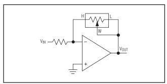
Figure 9. Variable Gain Inverting Amplifier
