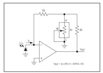
Figure 12. Variable Gain I-to-V Converter
