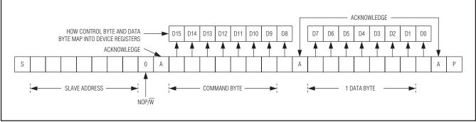
Figure 7. Command and Single Data Byte Received
