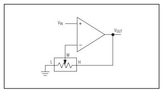
Figure 8. Variable Gain Noninverting Amplifier
