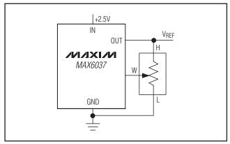
Figure 11. Adjustable Voltage Reference
