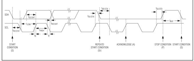
Figure 2. I<sup>2</sup>C Serial-Interface Timing Diagram
