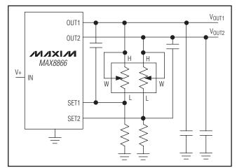
Figure 10. Adjustable Dual Linear Regulator
