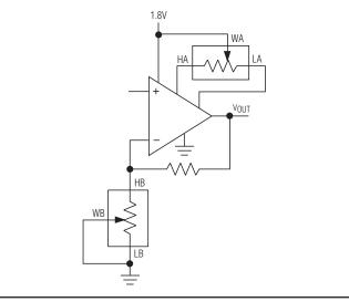
Figure 15. Programmable Filter
