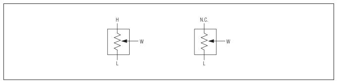
Figure 1. Voltage-Divider and Variable Resistor Configurations
