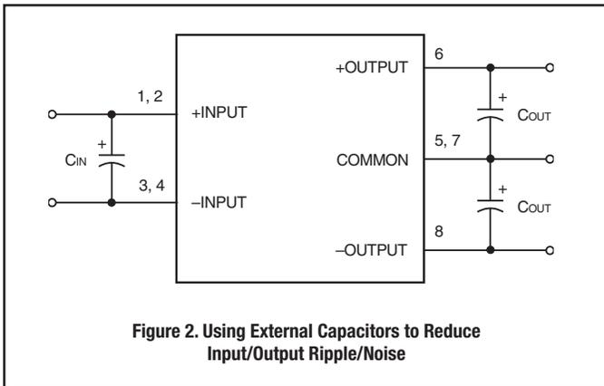
**Figure 2. Using External Capacitors to Reduce Input/Output Ripple/Noise**
