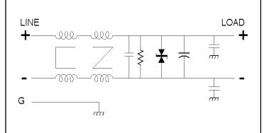
Operating Voltage = \_\_\_\_\_100 Vdc Operating Current MAX = \_\_\_\_\_1 Amp Temperature Range = \_\_\_\_\_-20 to  $50\,^{\circ}$ C Dielectric Withstand (L-Grd), 1 Min = \_\_\_\_\_1500 Vac Calculated MTBF = \_\_\_\_\_8,081,461 Hrs @ 300176C GB
