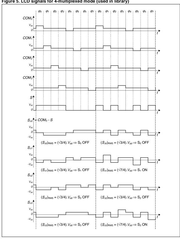
Figure 5. LCD signals for 4-multiplexed mode (used in library)
