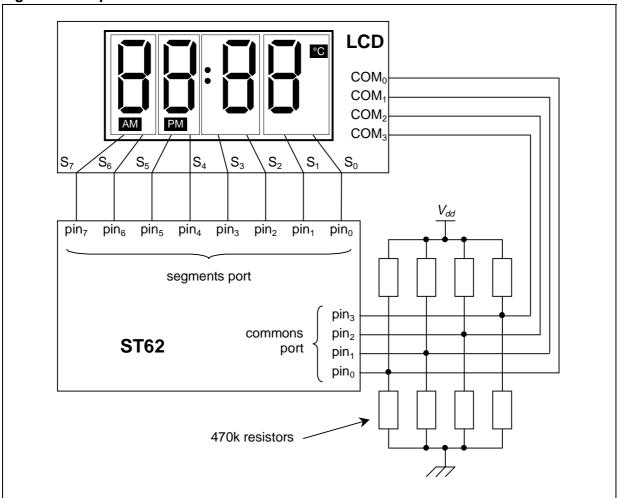
Figure 7. Template for MCU – LCD connections
