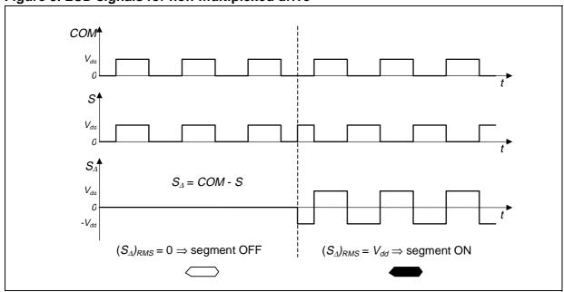
Figure 3. LCD signals for non-multiplexed drive
