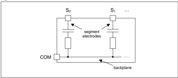
Figure 2. Connections inside a direct drive LCD
