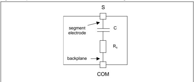
If no voltage is applied to it, a segment is transparent. To make it opaque, the LCD driver must apply an AC voltage which Root Mean Square (RMS) value is above a certain threshold. This voltage threshold depends on the LCD characteristics.
