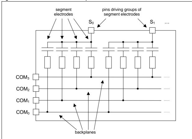
Figure 4. Connections inside a 4-multiplexed LCD
