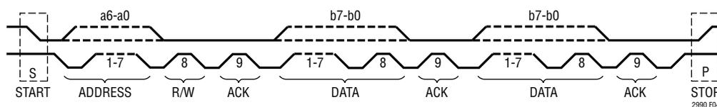
Figure 4. Data Transfer Over I<sup>2</sup>C or SMBus
