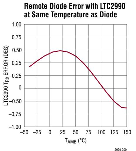
**TYPICAL PERFORMANCE CHARACTERISTICS**  $T_A = 25^\circ\text{C}$ ,  $V_{CC} = 3.3\text{V}$  unless otherwise noted
