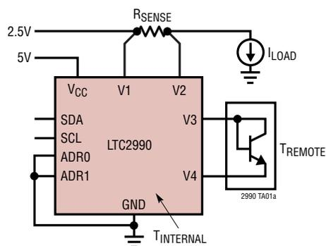
MEASURES: TWO SUPPLY VOLTAGES, SUPPLY CURRENT, INTERNAL AND REMOTE TEMPERATURES
