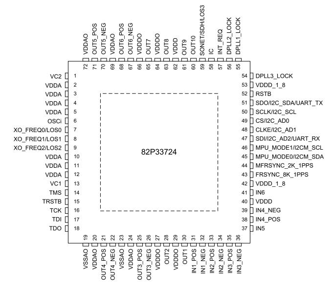
Figure 2. Pin Assignment (Top View)
