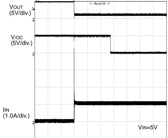
Figure 37. Over-Current Response 1Ω Load Connected at Enable
