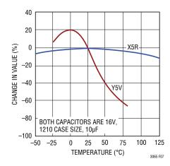
Figure 7. Ceramic Capacitor Temperature Characteristics
