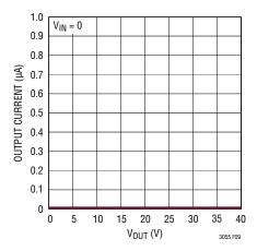
Figure 9. Reverse Output Current
