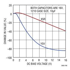
Figure 6. Ceramic Capacitor DC Bias Characteristics
