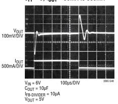
**5V Transient Response**  $C_{FF} = 10nF$ ,  $I_{OUT} = 50mA$  to 500mA
