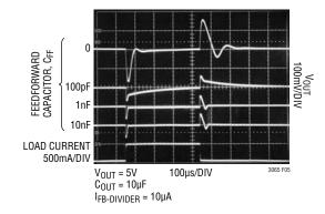
Figure 5. Transient Response vs Feedforward Capacitor
