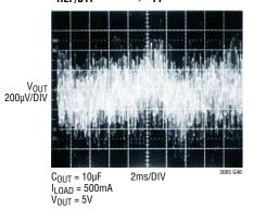
10Hz to 100kHz Output Noise  $C_{REF/BYP} = 10nF$ ,  $C_{FF} = 10nF$
