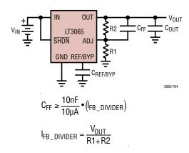
Figure 4. Feedforward Capacitor for Fast Transient Response
