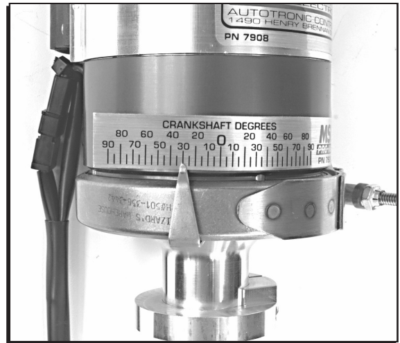
Figure 6 Applying the Timing Tape.
