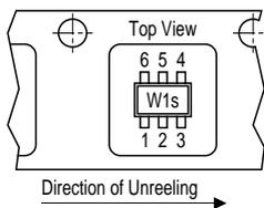
Marking on SC74 package (for example W1s) corresponds to pin 1 of device
