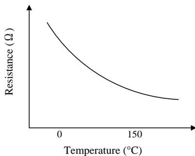
Figure 6-2 Reference characteristics of NTC thermistor
