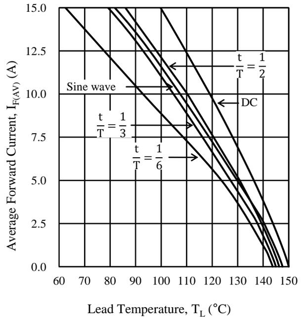
Figure 3-19  $I_{F(AV)} - T_L$  ( $V_R = 200\text{ V}$ )
