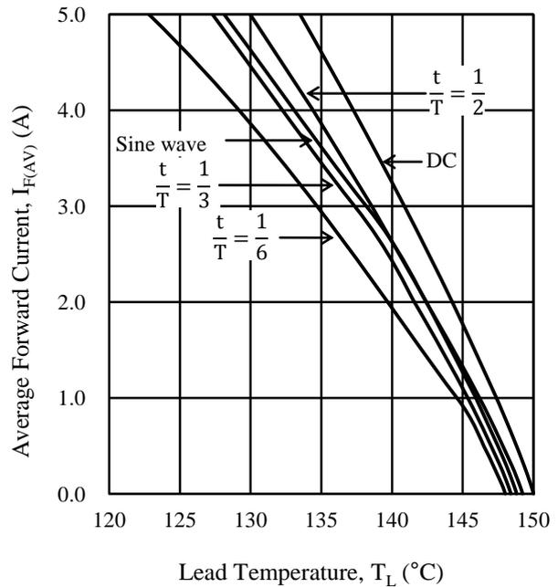
Figure 3-7  $I_{F(AV)} - T_L (V_R = 200\text{ V})$
