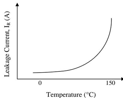
Figure 6-4 Reference temperature characteristics of SBD leakage current
