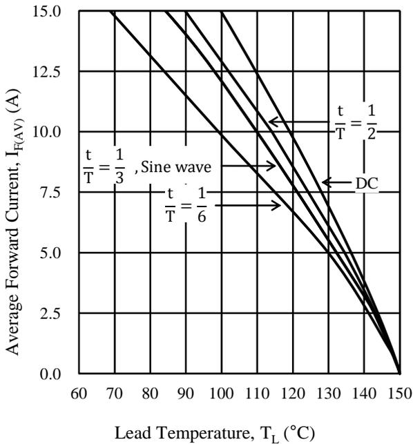
Figure 3-18  $I_{F(AV)} - T_L$  ( $V_R = 0\text{ V}$ )
