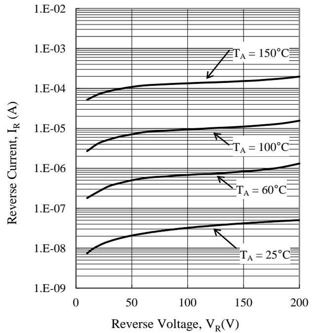
Figure 3-3  $I_R - V_R$  Typical Characteristics
