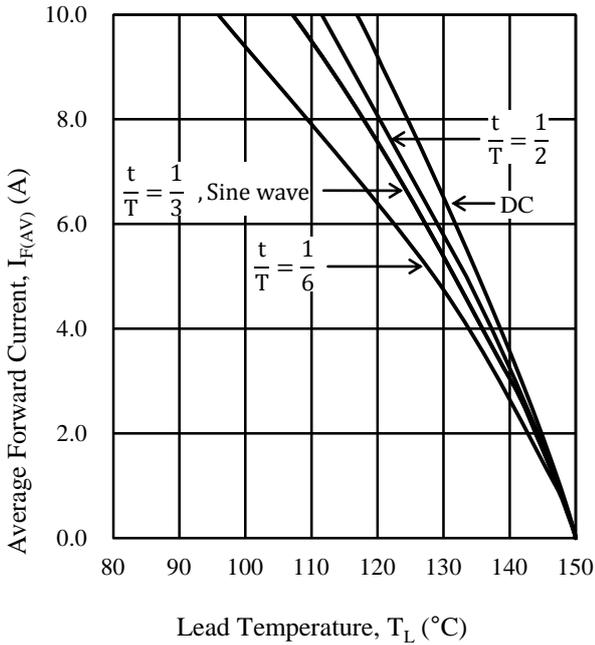
Figure 3-12  $I_{F(AV)} - T_L$  ( $V_R = 0\text{ V}$ )
