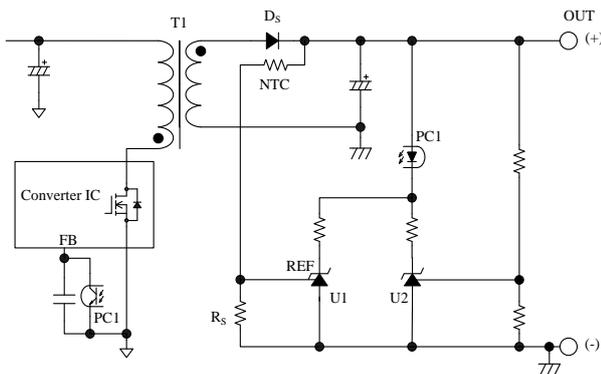
Figure 6-1 Reference temperature detection circuit with NTC thermistor
