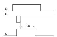
1) The terminal 30 is connected with positive electrode of power supply, terminal 87 is connected with load, the terminal 86 is connected with nature, the terminal 85 is connected with control signal. As shown in logic diagram, the terminal 30 and 87 will be connected when terminal 85 received a low level start-up signal, the terminal 30 and 87 will be opened when 85 terminal start-up signal disappeared and delayed 9s±2s.
