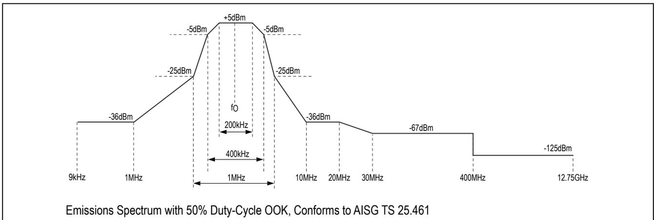
Figure 3. AISG Standard Modem Spectrum Emission Mask
