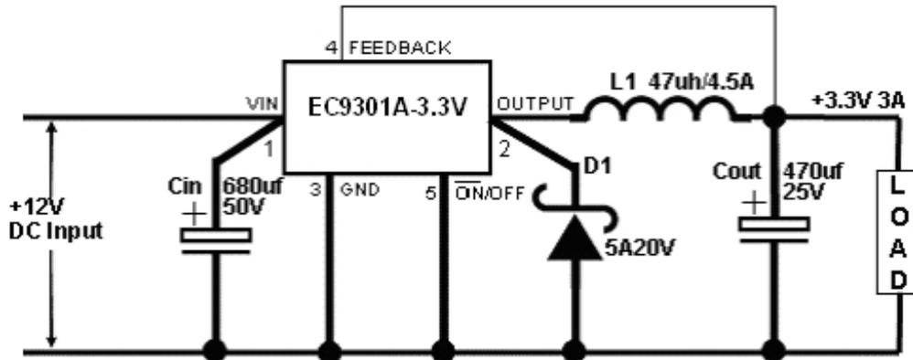
Figure 11. Typical Application of EC9301A For 3.3V
