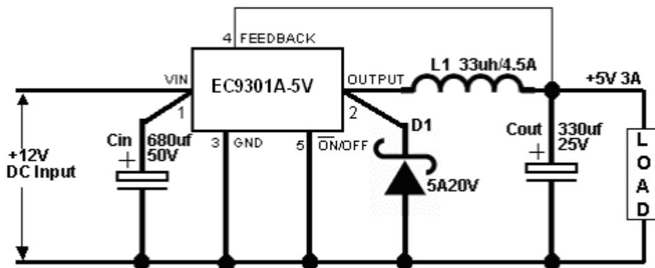
Figure 12. Typical Application of EC9301A For 5V
