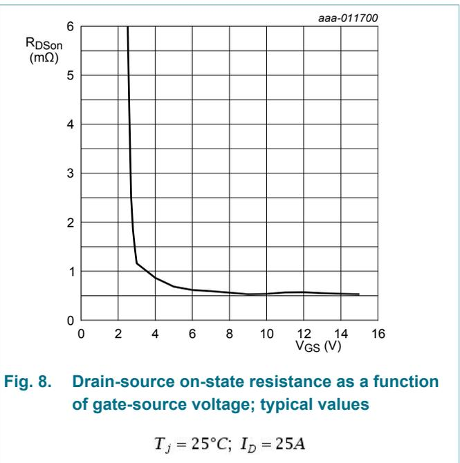
N-channel 30 V, 0.87 mΩ logic level MOSFET in LPAK56 using NextPowerS3 Technology
