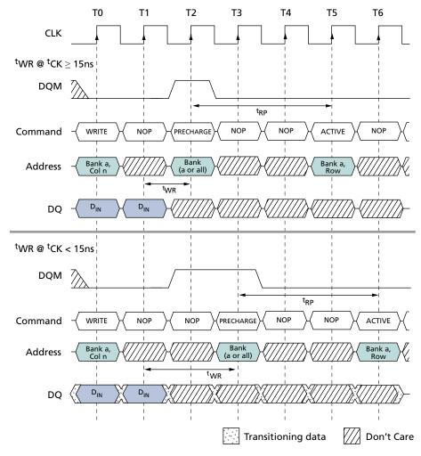
Note: 1. In this example DQM could remain LOW if the WRITE burst is a fixed length of two.
