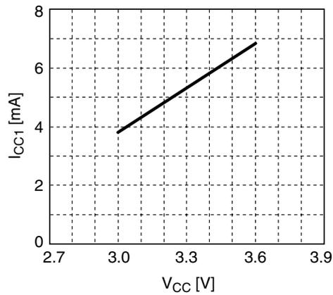
Figure 1. Current consumption 1 vs. Supply voltage
