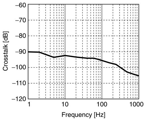
Figure 9. Crosstalk vs. Frequency\*<sup>3</sup>
