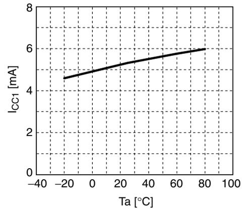
Figure 2. Current consumption 1 vs. Ambient temperature
