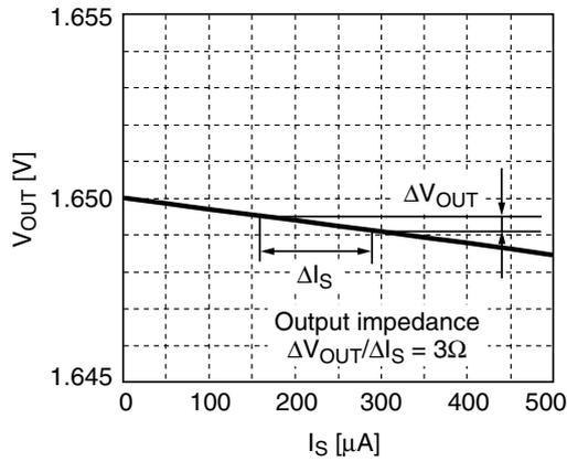
Figure 7. Output current vs. Output voltage\*<sup>1</sup>
