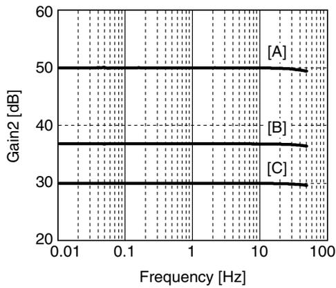
Figure 6. Output gain vs. Frequency (when changing output gain setting<sup>\*1</sup>)
