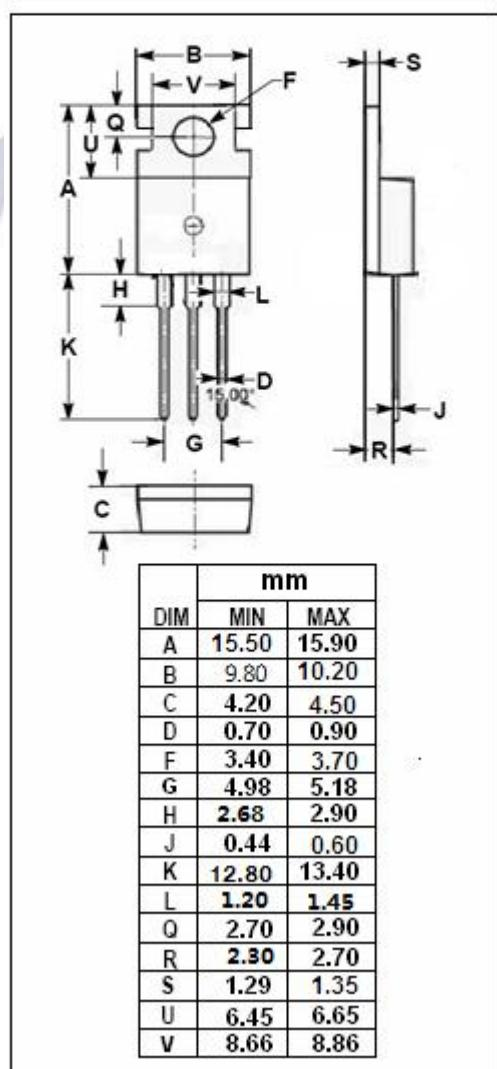
**isc N-Channel MOSFET Transistor****60N06-18****• ELECTRICAL CHARACTERISTICS ( $T_c=25^\circ\text{C}$ )**
