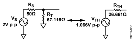
Figure 48. Thevenin Equivalent Circuit
