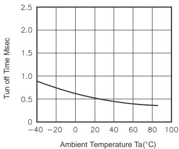
**Fig.5** LED operate vs. ambient temperature
