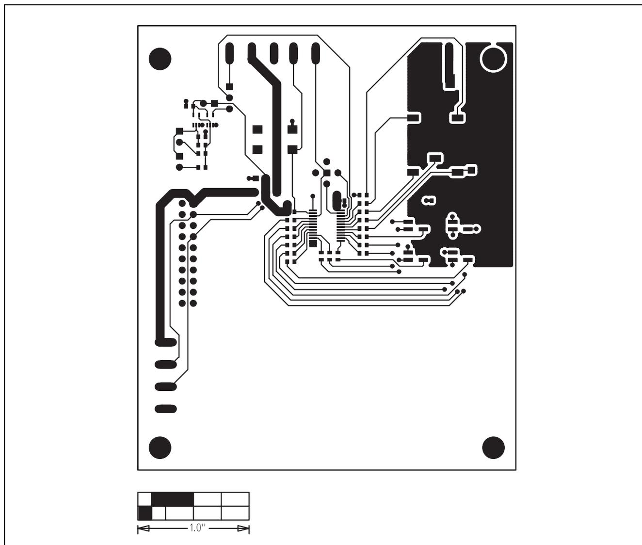
Figure 6. MAX6964 EV Kit PCB Layout—Component Side
