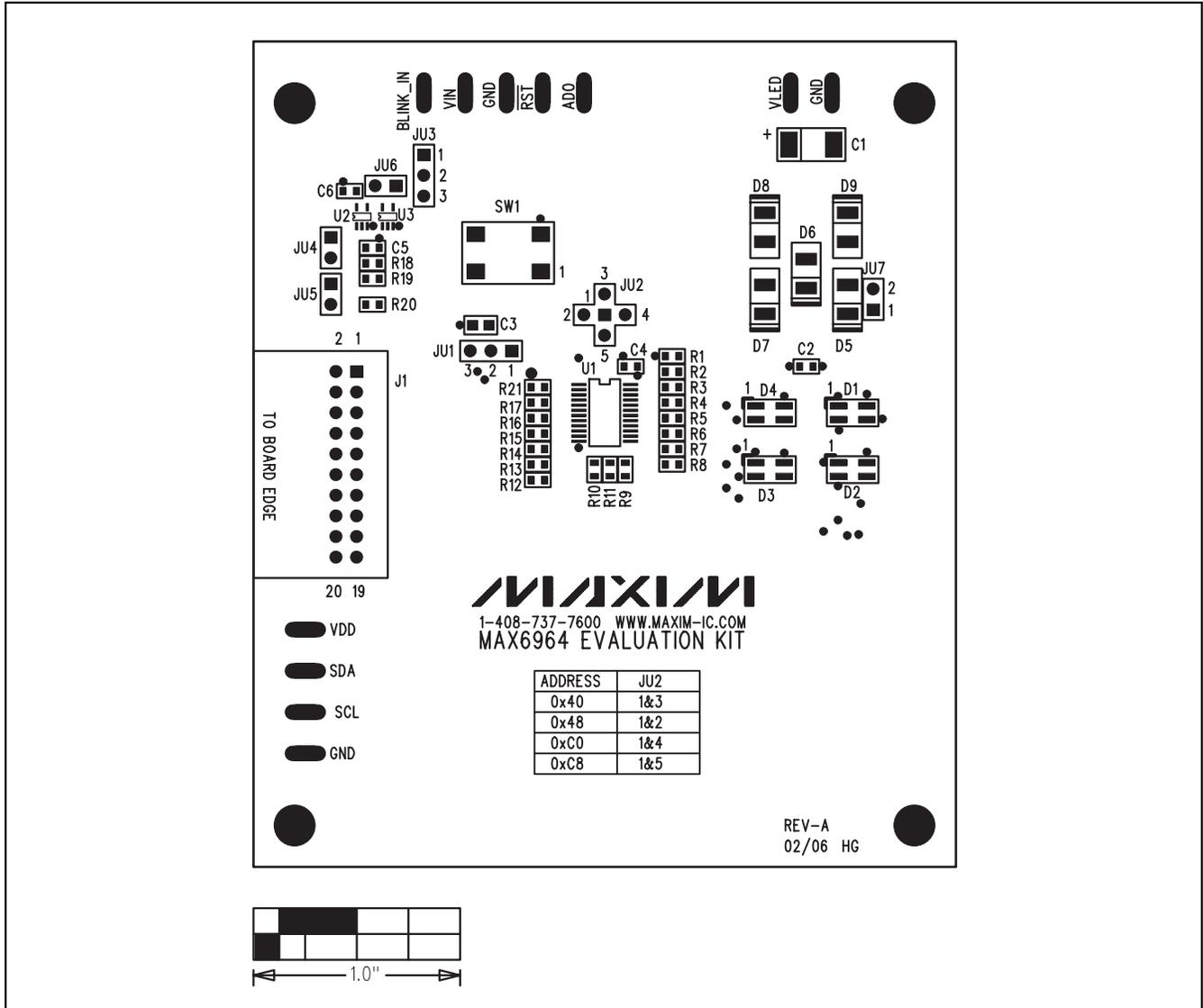
Figure 5. MAX6964 EV Kit Component Placement Guide—Component Side
