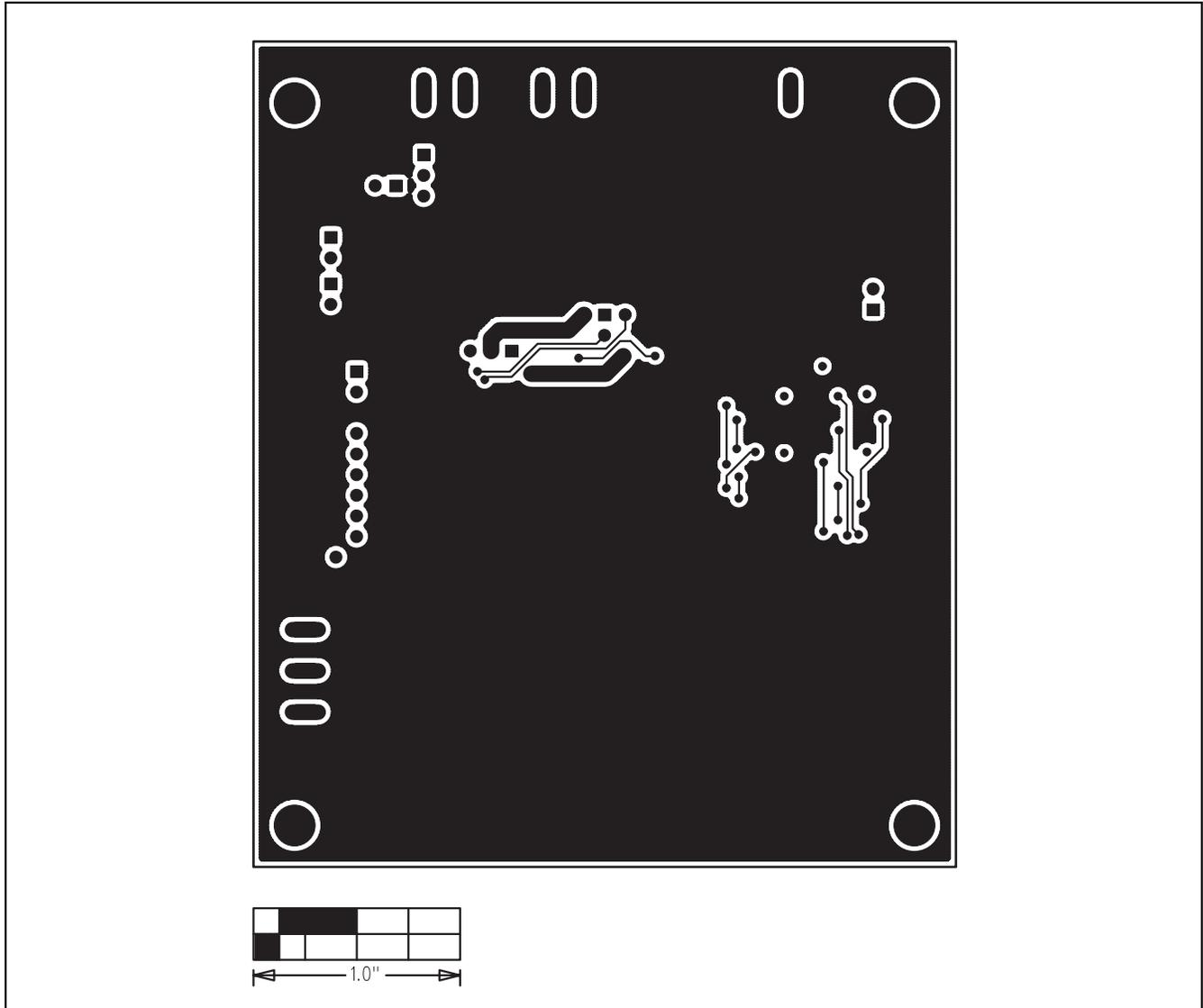
Figure 7. MAX6964 EV Kit PCB Layout—Solder Side
