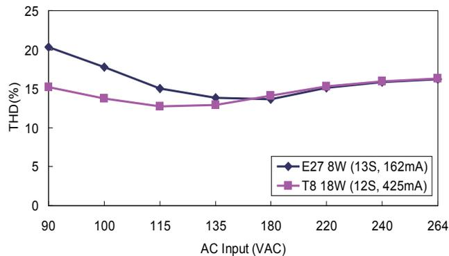
Figure 14. E27/T8 THD vs. Wide AC Voltage
