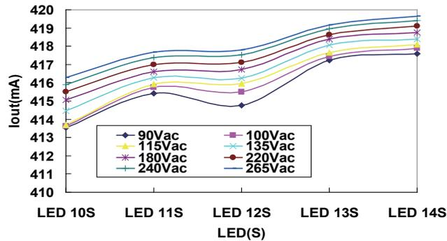
Figure 10. Iout vs. LED(s) Regulation in T8 Tube
