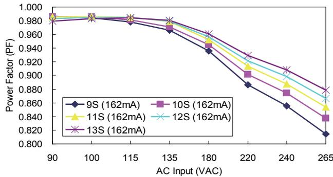
Figure 9. Power Factor (PF) vs. Wide AC Voltage in E27(8W, 13S / 162mA) Bulb
