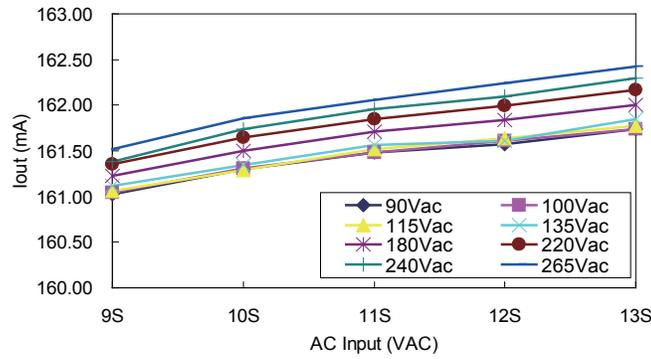
Figure 6. Iout vs. LED(s) Regulation in E27 Bulb
