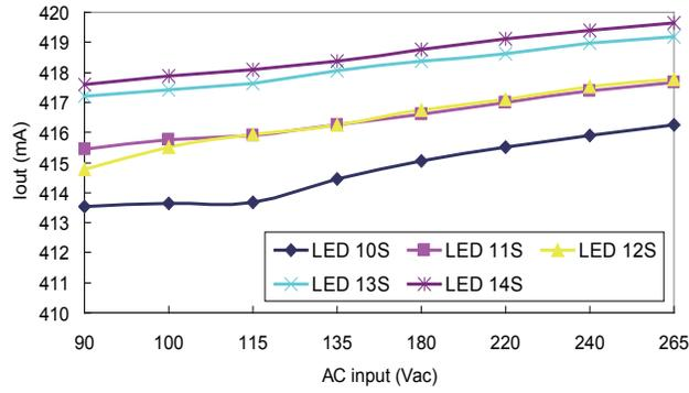
Figure 11. I<sub>out</sub> vs. Wide AC Voltage in T8 (18W, 12S / 425mA\*) Tube
