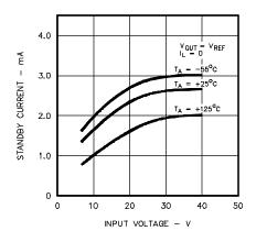
Figure 5. Standby Current Drain
