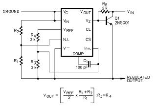
Figure 10 - Negative Voltage Regulator
