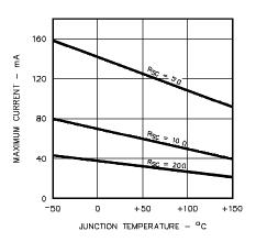
Figure 3. Current Limiting Characteristics
