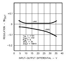
Figure 4. Regulations vs. Input-Output Voltage Regulation
