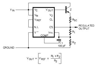
Figure 9 - High Current Regulator External NPN Transistor  $I_1 = 1.0 \text{ A}$
