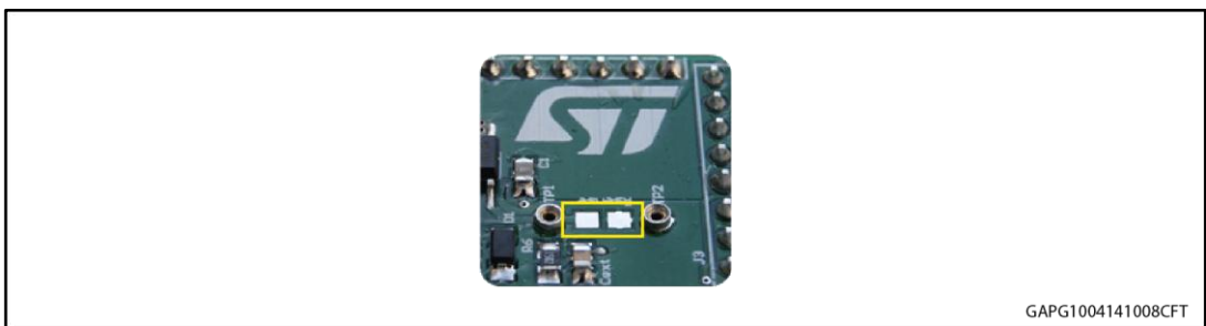
Figure 5: Pads for soldering SMD resistor
