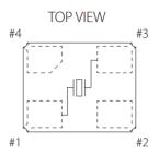
• #1,#3 : Crystal terminal / #2,#4 : Connected to cover (Please connect it with GND.)
