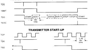
$Upon da: a transmission initiation, or when not transmitting at 100\% line utilization, the start bit will be placed on the TSO line at the high to low transition of the TCP clock following the trailing edge of <math>\overline{\text{TDS}}$ .
