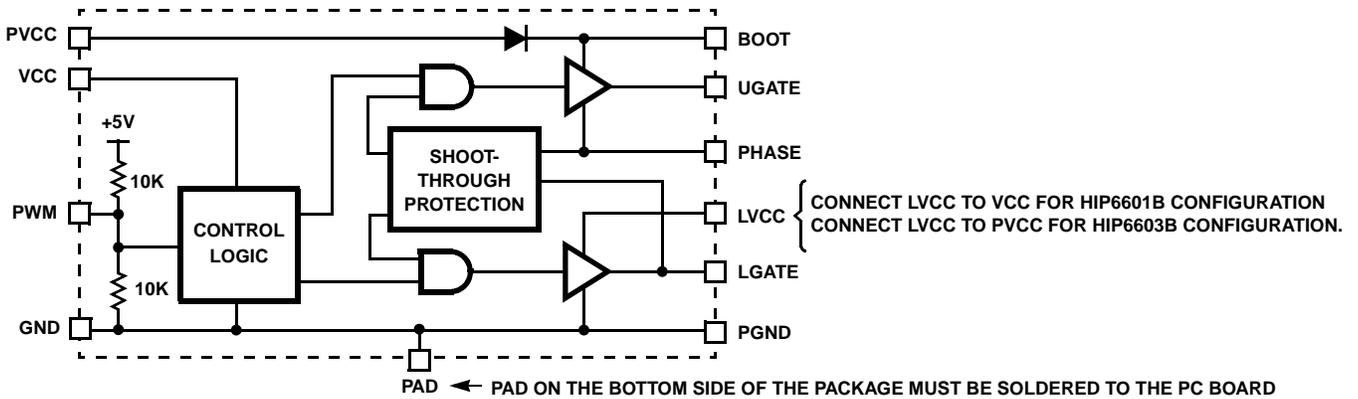
Typical Application: 3-Channel Converter Using HIP6301 and HIP6601B Gate Drivers
