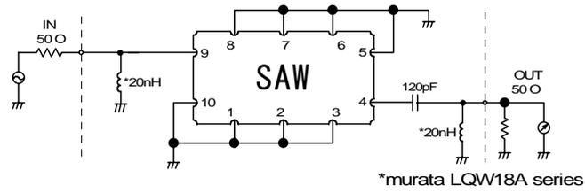
Fig.1 Measuring circuit
