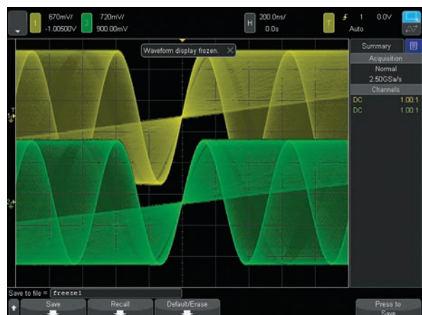
Figure 44. The "freeze screen" feature keeps the intensity-grading information while stopping the waveform acquisition.
