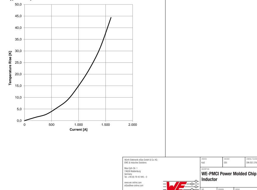
**Typical Temperature Rise vs. Current Characteristics:**
