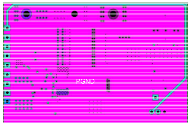
Figure 35f: IRDC1827 demoboard layout considerations – Mid Layer 4
