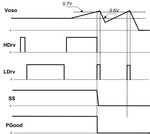
Figure 12b: iP1827 Signal Timing for OVP
