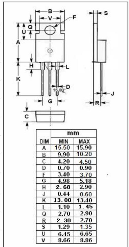
**isc N-Channel MOSFET Transistor**
