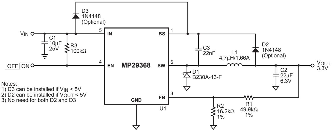
**Figure 3—1.4MHz, 3.3V Output at 1A Step-Down Converter**
