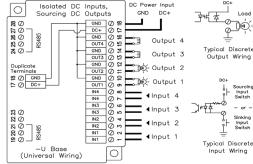
Connect up to 4 DC Outputs and 4 Externally Powered DC Inputs
