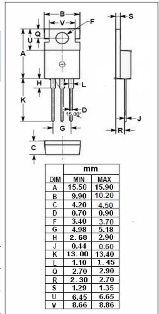
**isc N-Channel MOSFET Transistor**
