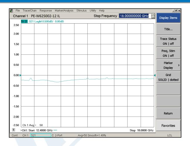
Click the following link (or enter part number in "SEARCH" on website) to obtain additional part information including price, inventory and certifications: WR-62 Instrumentation Grade Straight Waveguide Section 12 Inch Length with UG-419/U Flange Operating from 12.4 GHz to 18 GHz PE-W62S002-12
