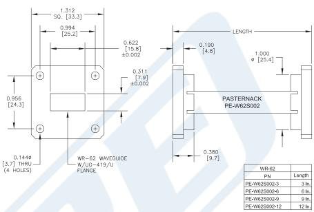
WR-62 Instrumentation Grade Straight Waveguide Section 12 Inch Length with UG-419/U Flange Operating from 12.4 GHz to 18 GHz from Pasternack Enterprises has same day shipment for domestic and International orders. Our RF, microwave and millimeter wave products maintain a 99% availability and are part of the broadest selection in the industry.
