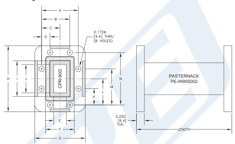
WR-90 Commercial Grade Straight Waveguide Section 12 Inch Length with CPR-90G Flange Operating from 8.2 GHz to 12.4 GHz from Pasternack Enterprises has same day shipment for domestic and International orders. Our RF, microwave and millimeter wave products maintain a 99% availability and are part of the broadest selection in the industry.
