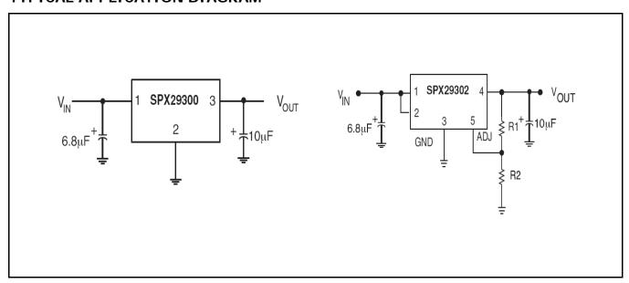
Fig. 1: SPX29300 and SPX29302 Application Diagrams
