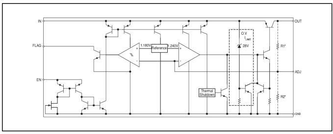
Fig. 2: SPX29300/01/02 Block Diagram
