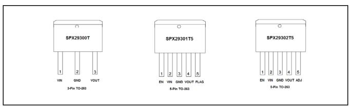
Fig. 3: SPX29300/01/02 Pin Assignment
