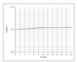
Fig. 6: Line Regulation  $I_{OUT}=10mA$ ,  $V_{OUT}=3.3V$
