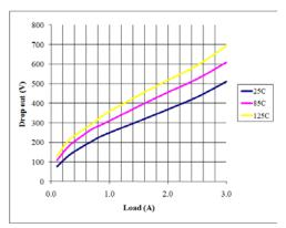
Fig. 4: Dropout Voltage vs Load Current
