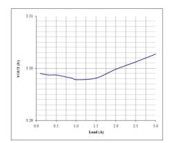
Fig. 7: Load Regulation  $V_{OUT}=3.3V$
