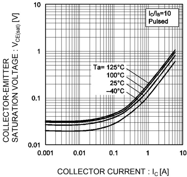
Fig.6 Collector-Emitter Saturation Voltage vs. Collector Current (II)
