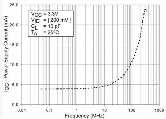
**Figure 8. Power Supply Current vs. Frequency**
