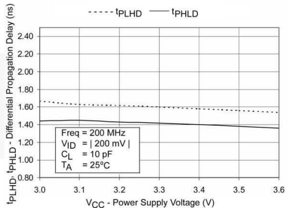
**Figure 10. Differential Propagation Delay Power Supply Voltage**
