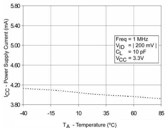
**Figure 9. Power Supply Current vs. Ambient Temperature**
