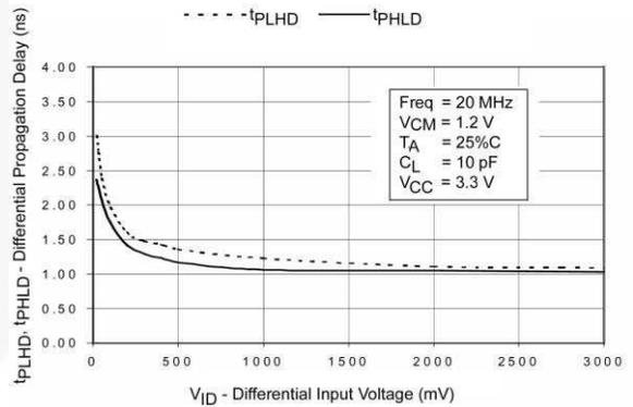
**Figure 14. Differential Propagation Delay vs. Differential Input Voltage**
