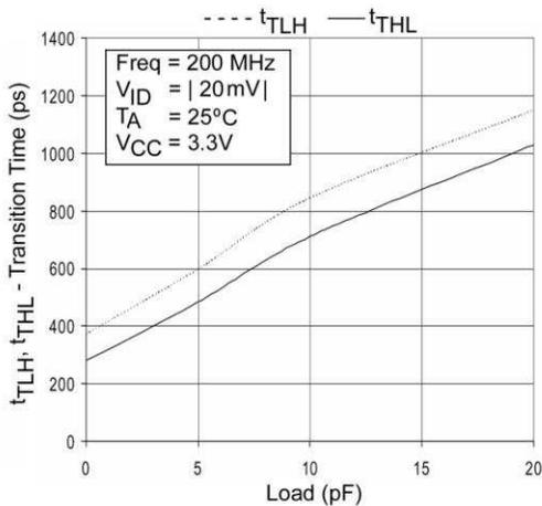
Figure 21. Transition Time vs. Load
