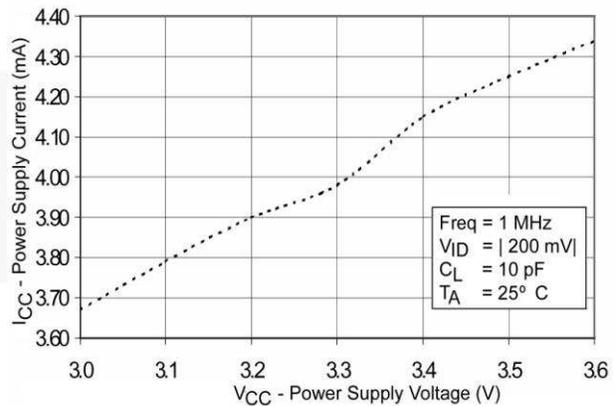
Figure 22. Power Supply Current vs. Power Supply Voltage
