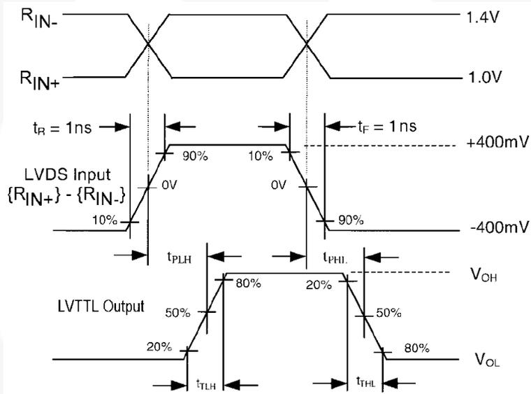
**Figure 4. LVDS Input to LVTTTL Output AC Waveforms**
