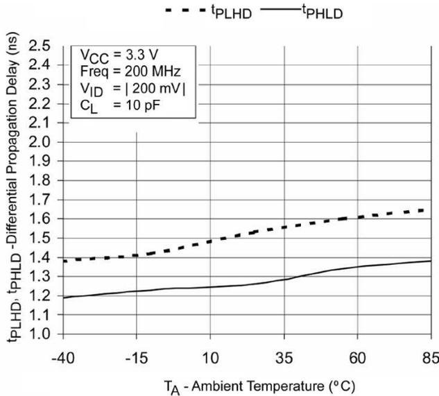
**Figure 11. Differential Propagation Delay vs. Ambient Temperature**
