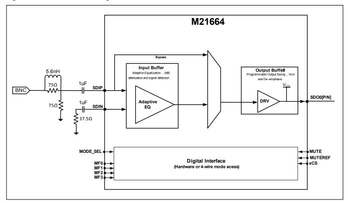
Figure 4-2. M21664 Block Diagram
