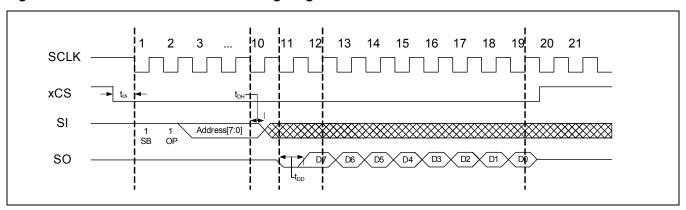
Figure 4-7. 4-wire Sequential READ Timing Diagram
