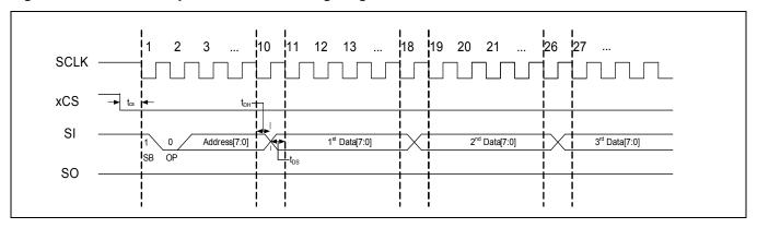
Figure 4-6. 4-wire Random READ Timing Diagram
